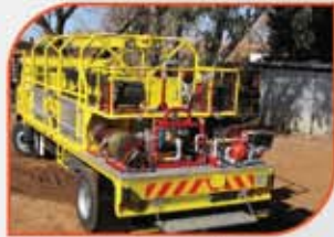
Forestry type heavy duty pumper
